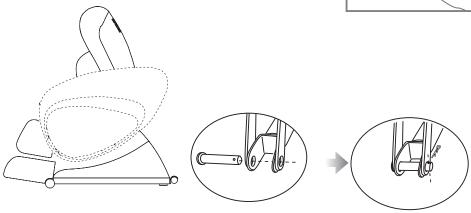
Connect and lock backrest to bottom seat then secure position.
