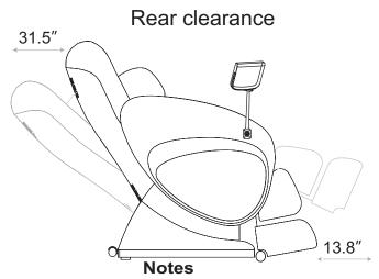
Allow for at least 31.5" rear clearance behind and the chair and 13.8" in font of the chair when installing.
